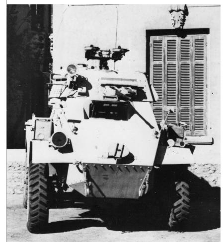
Above: Two views of Humber Armored Car(s) Mk III one of which is fitted with twin Vickers machine guns. Remarks: The Mk III was the essentially an improved Humber AC Mk II with the
