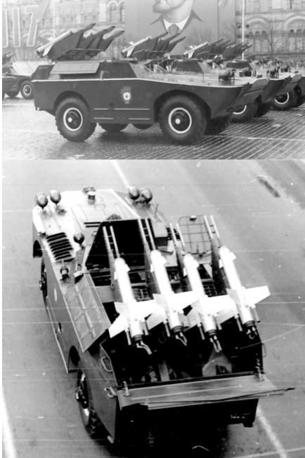
Above and top: Soviet/Russian 2P32 missile carriers. Fitted with powered (non-armored) cover panels, the top could also be supplemented with a tarp to keep out the weather. (Photos: Author's collection)
