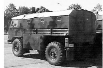
Above: Two views of the TAM 110 Ris (Lynx) Armored Personnel Carrier. The vehicle can be fitted with a light or heavy machine gun and firing ports are supplied under the side vision windows, a separate firing port is also available under the right hand windshield. (Photos Tovama Avtomobilov Motorjev [TAM])
