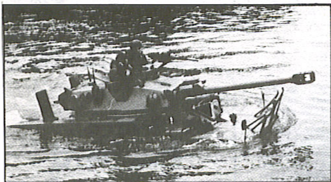
Panhard ERC swimming, using its two hydrojets. Note the engine compartment ducts in the raised position.
