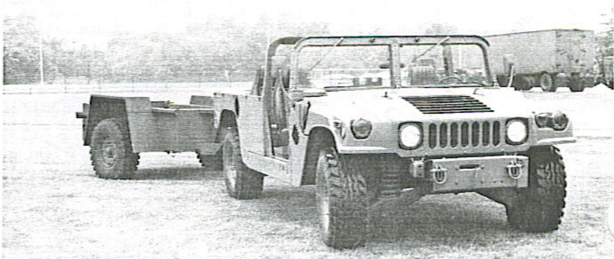
Three-quarter view of the Desert Mobility Vehicle System (DMVS) modified HMMWV and fabricated trailer.
