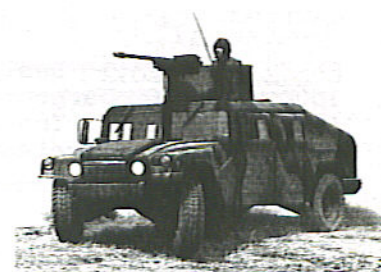
UP-ARMORED HUMMER shown here with McDonnell Douglas Helicopter Company's 30mm ASP-30 ® Cannon.
