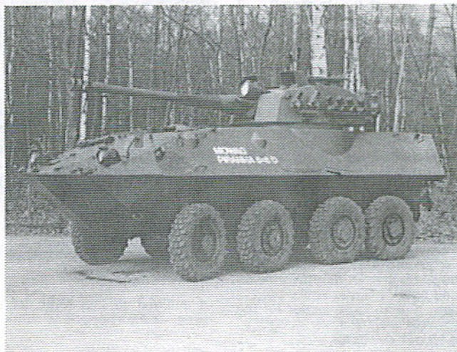
Above: 8 x 8 D with 90mm Cockrill turret. Photo: MOWAG AG.
