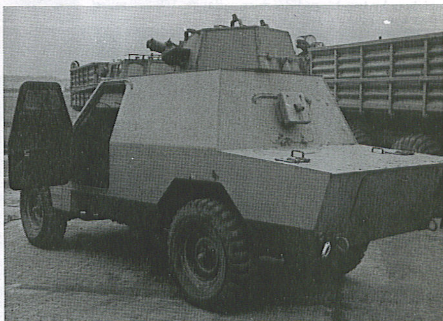
Top: Right side of a Shorland Mk III Series III, armored car, which is missing its turret armament as well as military registration plates. This vehicle shows the external recognition features such as recessed head lights and full-width wire mesh grill of the Mk III. During the mid-1980's Shorlands' such as this one, were sold to civilians (this sample belonged to the Budge Collection). Bottom: View from the rear with the crew escape hatch, and a lower hatch giving access to a storage compartment. Photos © Jochen Vollert.
