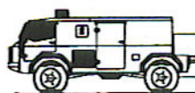
ARMoured BOMB DISPOSAL (EOD) Side ramp remotely deployed robot. Rear extra heavy 'bomb blast' wall. Rear mounted 'bomb tub'. Crew of 2.
