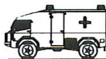
ARMoured AMBULANCE 4 stretcher patients, driver, commander and 2 medical orderlies. High roof for medical orderlies to stand.
