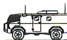
ARMoured COMMAND Separate rear-mounted generator to power communications equipment. Powered antenna masts.
