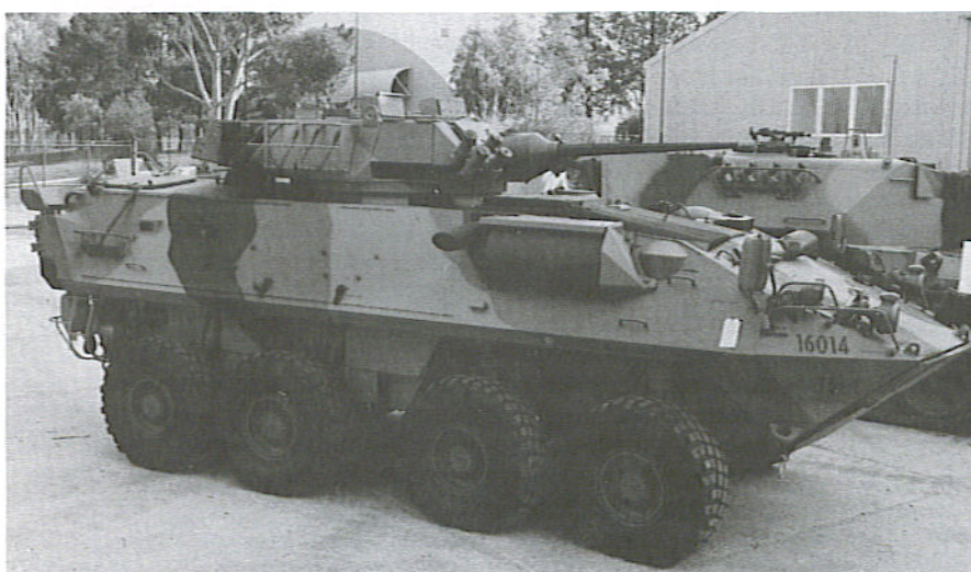
Brand new ASLAV with 25mm turret and all modifications in place photographed in 1995. Photo: Barry Marriott.
