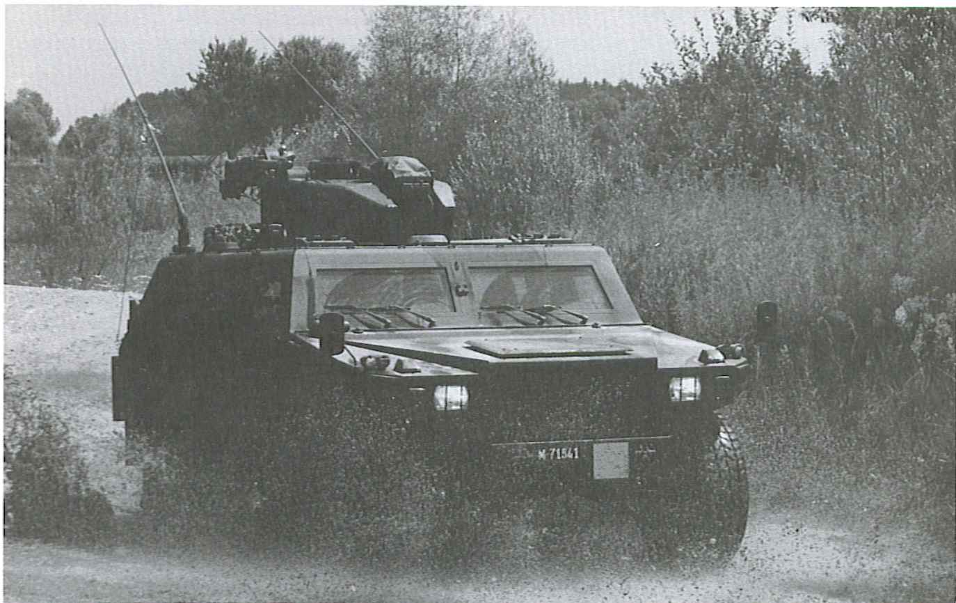
Right: MOWAG Eagle MBK2 turret. Below: Eagle during trials, the 7.62mm machinegun is mounted on the turret's right side, while the protective cover for the observation sight is in the closed position. Photo/Drawing: MOWAG Motorwagenfabrik AG.
