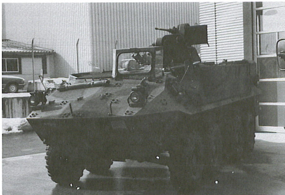
Above: Piranha II (8x8) APC with Kuka 606A1-CH .50 caliber turret and new external storage lockers. Photo: Raymond Surlémont.
