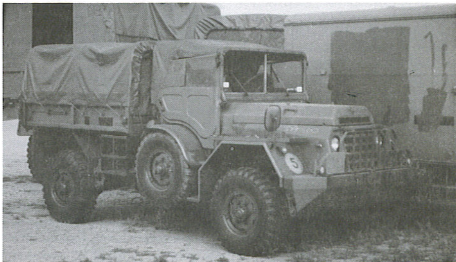
Above right: DAF YA-126, the chassis of which was used as the basis of the YP-104 Scoutcar. Photo: H. Heesakkers. Below: Left side of the YP-104 prototype, with the original three storage bins and space for extra fuel cans. The vehicle has a strong resemblance to the Daimler Ferret. Photo: DAF, via H. Heesakkers
