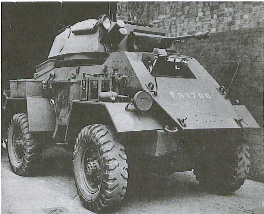
Above: Armored Car, Humber Mk III, just finished being overhauled and refitted. Photo: D.R. Haugh, Collection.
