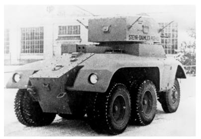
Remarks: Only two or three ADKZs were completed, with no series production by Styer-Daimler-Puch. A straight forward design, the vehicle had the driver at the front, engine at the rear and all-wheel drive. The weapons carried were, for the time substantial, with both a 20mm cannon and 8mm heavy machinegun in the turret. The final version had a frame radio antenna and curved fenders.
