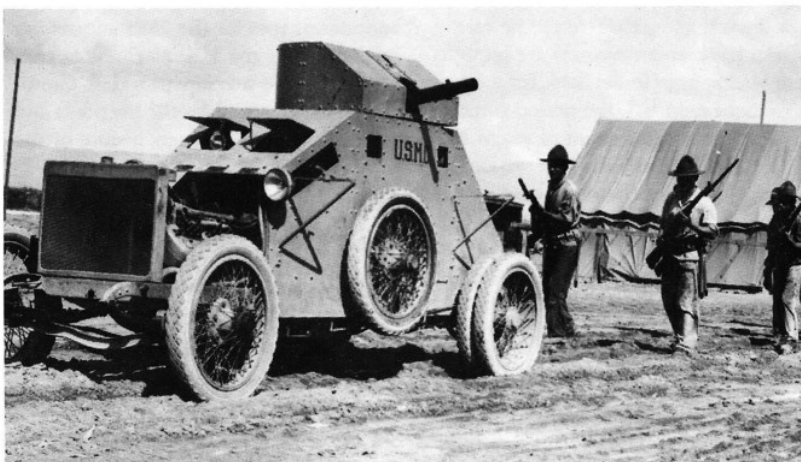
King of the 1st Armored Car Squadron with Marines in an anti-riot wedge in Haiti. The armor for the radiator and motor has been removed to reduce tropical cooling problems. The term "squadron" reflects the intended reconnaissance role for the cars.
