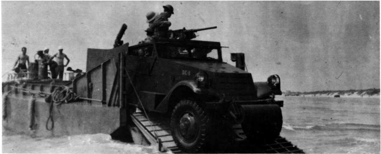
M3A1 scout car landing from an LCM-6, circa 1941. The M3 and motorcycles with sidecars equipped the 1st and 3d Scout Companies of the 1st and 2d Marine Divisions, until jungle operations on small Pacific islands made their use impractical. The scout companies were in the South Pacific in early 1942 but when the divisions moved north the cars were left in New Zealand.
