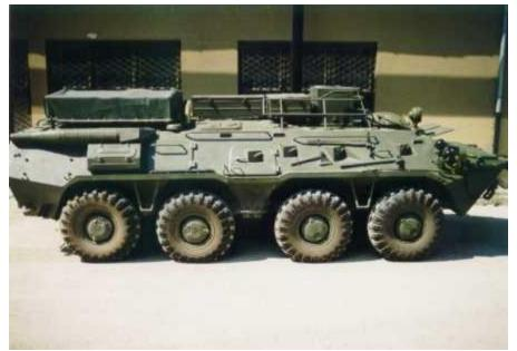
The BTR-80 MPAEJ (Technical Barrier Armored Response Vehicle) has a primary function of the reconnaissance of artificial barriers, devastated ground and the removal of such barriers. It is also designed to have a secondary mission of the protected movement of specialist personnel and their equipment.
