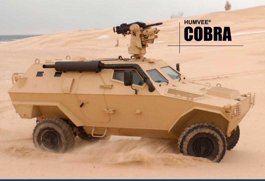
MONOCOQUE CONSTRUCTION / V-SHAPED HULL / HUMVEE DRIVE TRAIN COMPONENTS / AIR CONDITIONED
