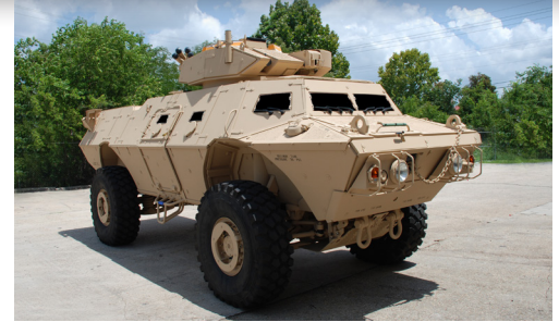
Along with the 40mm/.50 cal turret (above) and the gunner's protection kit, other options are available.
