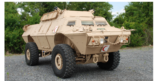
The APC ambulance provides ballistic and blast protection to the medical crew during patient treatment and transport.
