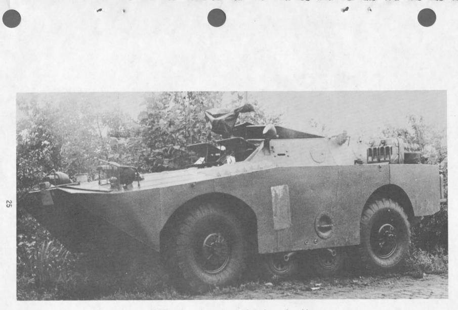
BRDM with rough terrain wheels in lowered position.
