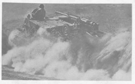
OT-62B with 82mm recoilless gun mounted on rear deck.
