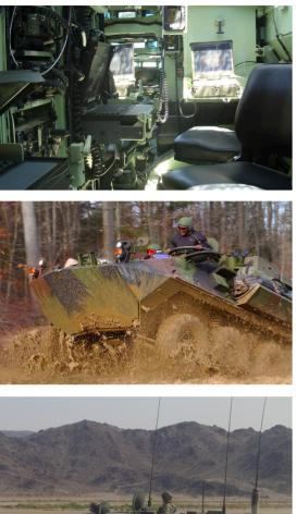
The U.S. Marine Corps Light Armored Vehicle-Command and Control is an improved LAV-25 with new communication and digital battlefield management systems that improve voice and data connectivity. The vehicle is an important enabler for fully informed intelligence, fire support and maneuvers during amphibious and land operations in a Light Armored Reconnaissance (LAR) battalion or independent LAR company units.
