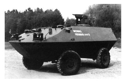
Remarks: A further development of the original 1972 version of the Piranha 4x4, the engine had been changed to a diesel and the transmission to an automatic. Fittings and parts were common to the other Piranha series. Although the weight had gone up the vehicle still had the same range and speed as the original design. The 4x4 APC version didn't find any users and remained a prototype only.
