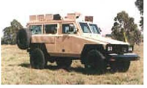
*Remarks*: The Mamba I, was designed by Dr. Vernon Joynt Mechem, using stock Toyota truck components for the engine and running gear. Primarily a police vehicle, the Mamba I was also used by the
