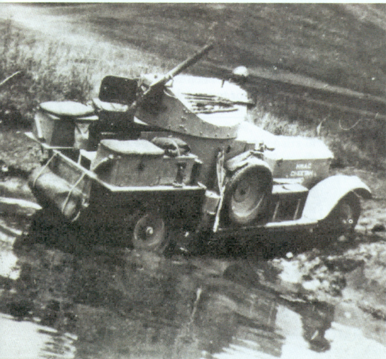
A very comprehensively kitted out armored Rolls-Royce fording a river. Note that the wheels now have solid metal discs.
