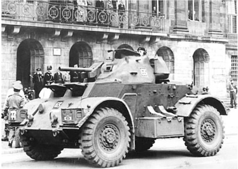
Above and left: T17E1 CS (Staghound II CS) in Europe. The larger 3-inch howitzer barrel shows clearly in the top picture as well as the blanked off bow machinegun position. (Photos: Author's Collection)
