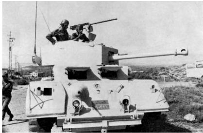
Remarks: By 1956 in addition to their standard 37mm armed T17E1 and 75mm armed Staghound Mk III armored cars, Lebanon had fielded a set of Staghounds with the turret replaced by that from the British AEC Mk III Heavy Armored Car. Like the Staghound Mk III. the vehicle was equipped with a 75mm cannon. It appears that no more than a dozen of these cars were completed with the last being retired in the early 1980's.
