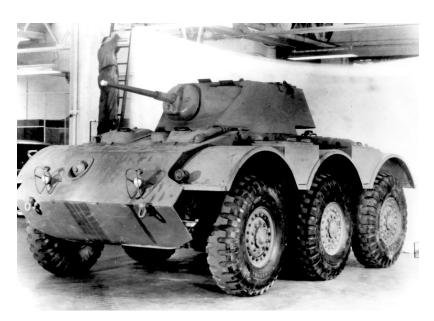
**Remarks**: Above, the second pilot T19, and the only T19E1. Modified and simplified from the original design, testing showed the vehicle was still too heavy for an efficient recon-naissance vehicle; although the chassis showed promise. At the request of Tank Destroyer Command, a 75mm gun M3 was mounted in an open turret and fitted to the chassis as the Carriage, Motor, 75-mm Gun, T66.
