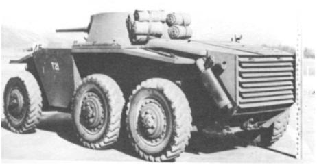
**Remarks:** Developed concurrently with the Ford T22 (which became the M8), the Studebaker T21 was a rear-engine design driving the rear two axles, making the car a 6x4. Had it been started earlier, the Studebaker design might have become standard, the Armored Vehicle Board judging the car satisfactory as a reconnaissance vehicle,
