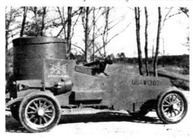
Remarks: Completed just prior to the Armored Car, T8, the T9 used a Plymouth chassis instead of one from Chevrolet. Performance and general appearance were much the same as well since both bodies were designed and built by the Holabird Quarter Master Depot in Maryland.
