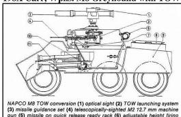
(9) diesel repower package (10) foot-operated machine gun firing pedal Remarks: At least six vehicles had the 37mm
