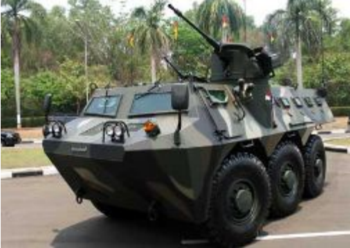
Above: The new PT Pindad APS-1 with 12.7mm turret. (Photo: PT Pindad)
