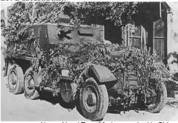
Above: Naval Type 92 photographed in China. **Data:** Weight of vehicle loaded, 13,600 lbs. (6,174 kgs). Armor, riveted steel plate. Suspension, Semi-elliptical spring. Transmission, manual. Drive, 6x4. *Armament:* (5) light machine guns and crew small arms. Crew, 5-6.
