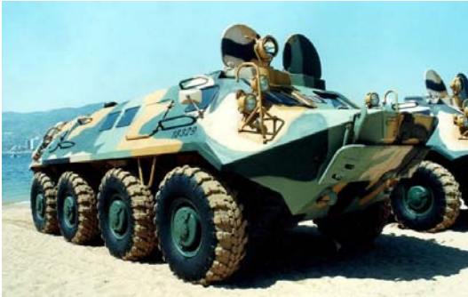
Above: Mexican Navy Marine APC-70. This vehicle is a modified Russian BTR-60 PB. (Photo: Photo: Armada de Mexico)
