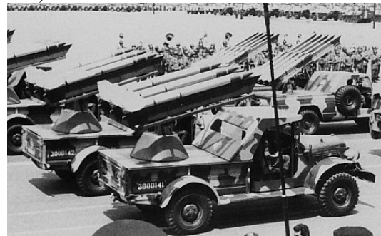
Above: M601 converted in Mexico to carry free flight rockets. (Photo: Author's Collection)
