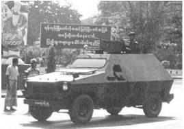
A locally produced armored car based on a commercial truck chassis with Nissan engine.
