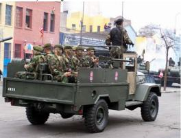
Above: Peruvian Army M-325 with "B" body set up as a personnel carrier with seats facing out and mounts for light machine guns. (Photo: Peruvian Army).
