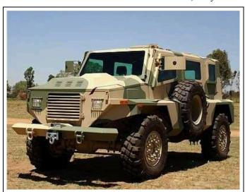
Oryx Data: Weight: Empty, 19,548 lbs (8875 kg). Length, 225 in (5716 mm). Width, 90.5 in (2300 mm). Height, 97.5 in (2477 mm). Ground Clearance, 14.5 in (366 mm). Wheel Base, 140 in (3555 mm). Drive, 4x4. Armor, armor /glass up to 7.62mm AP. Capacity: Fuel, diesel. Crew/Passengers,
