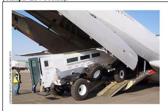
Above; Along with the Casspir-S, MECHEM developed a Casspir Mk II (New Build) that could operate with a lowered suspension. The new design is able to fit into most medium sized cargo aircraft; making deployment of a Casspir much easier. (Photo: MECHEM)
