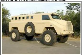
Remarks: Designed as a replacement for the aging Casspir series of mine-protected APCs, the Sable tried to build on the experience gained from years of field usage. The Sable is protected against up to a triple TM-57 AT mine (equal to 46 lbs [21 kg] of TNT) with the option of up-armoring against self-forming fragmentation mines. The monocoque hull is of steel construction with the vehicle commander and
