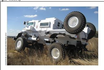
Above: Based on the Casspir Mk II (New Build) chassis and components the Casspir-S has a reduced armored crew compartment but with the addition of a tray at the rear capable to handle cargo or a weapon's mount. (Photo: MECHEM)
