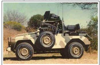
Above: CSIR G-BAT with 40mm Grenade launchers and personnel carrier pallet at the rear. (Photo: CSIR Technology)
