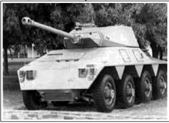
**Remarks**: This test-bed was built around a Saracen Armored Personnel Carrier (APC) side wishbone and torsion bar suspension and bevel box drive line system. The test-bed was built by Sandock Austral (Pty) Ltd in Boksburg circa 1979. The test-bed was to validate vehicle design features such as; suspension, soil mechanics, and large caliber gun firing stress mechanics. Firing trials were carried out with the muzzle brake fitted and removed from the 77mm cannon.
