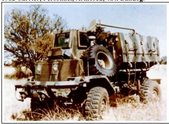
Remarks: Developed as a replacement for the Buffel armored personnel carrier, the new vehicle was based on the South African developed SAMIL 20 truck chassis. Like the Buffel, the Bulldog is open topped vehicle with the driver in a separate compartment at the front, and the crew carried in a blast resistant compartment at the rear of the vehicle. While the South African Army chose the Casspir as their new APC, the Air Force selected the Bulldog, and uses them for airfield defense.
