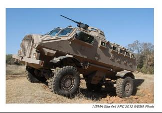
Above: In an effort to meet the demand for new vehicles similar to the Casspir, IVEMA has produced a near clone to the original vehicle. The vehicledoes feature a new engine and running gear, along with a redesigned interior. An Anti-Aircraft/Anti-Tank mounting as well as a Police/Interior Security design has also been developed. (Photo IVEMA)
