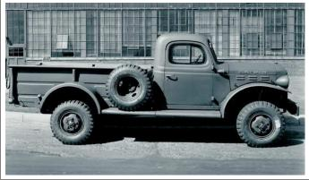
Above: Truck, Pickup, 1-ton, 4x4 (Dodge, Model B2PW126). **Remarks:** A civilian vehicle derived from the WC 3/4-ton trucks of WWII. Dodge used their experience to produce a 1-ton 4x4 truck capable of off-road service. With the US their aging WWII vehicles the Power Wagon was taken and bought directly from the factory (Usually as a chassis Vol/Weight, 68 cu ft (1.9 cu m) or 3,405 lbs (1546 kgs).
