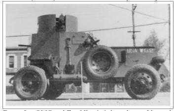
**Remarks:** QMC and Franklin, 4x4, interchangeable truck or armored bodies, 6 built. Armament (1) .50 caliber HMG and two .30 caliber light machine guns. Engine, Franklin 6-cyl. This car had an unloaded weight of 7,200
