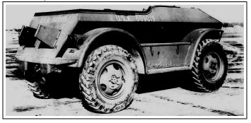
with the addition of an armored, open topped body, no production undertaken, circa 1941-42.
