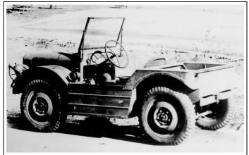
Above: Chevrolet Extra Light at Aberdeen Proving Ground. Remarks: Two vehicles of the same design were completed by Chevrolet for the 1943 extra-light vehicle requirement, but only one vehicle was actually tested.
