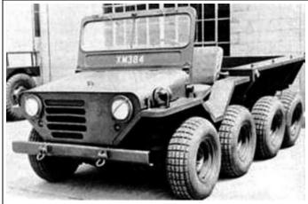
Vehicle Data: Length: 160 in (4064 mm). Width: 74 in. (1880 mm). Weight empty: 3590 lbs. (1630 kgs.). Payload: 2400 lbs. (1089.5 kgs.). Engine: Gasoline, 4-cyl, 70 hp (51.7 kW). Transmission: Manual, 4F-1R. Tire size: 7.10 x 15.
