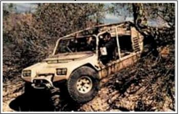
Remarks: Designed to fit the US Army's then current requirement for a Combat Support Vehicle (CSV). A rear engine design, development was halted in favor of the front engined HMMWV requirement.
