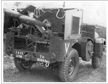
Above: M38A1 fitted with three French SS10 Anti-tank Missiles. **Remarks:** The SS-10 missle system was only in service with the US Army for approximately three years being replaced in 1963 by the ENTAC missile system.
