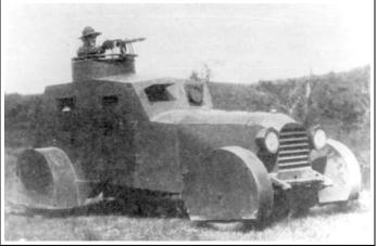
Remarks: An independent project, the 112th Cavalry vehicle was designed and built by Cpt. John B. Dunlap. Armament: (1) .30 cal. machine gun. Elevation, manual. Traverse, 360 degrees. Crew, 3-4. Engine: Type, gasoline. Location, forward. Cooling, liquid. Transmission: Type, manual. Suspension System: Type, leaf spring. Steering, front axle. No of wheels, 4. Performance: Speed/Land, 70 mph (112 km/h). Drive, 4x2. Usage: US Army, trial vehicle only.
