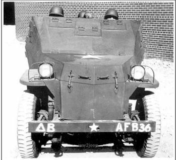
Above: T25E2 showing its small size, but well angled armor. **Remarks:** This was a further project of the T25 series to provide a light armored reconnaissance vehicle by adding 985 lb. of armor. The project was also terminated in Sep 1943 as being overload for the chassis.
