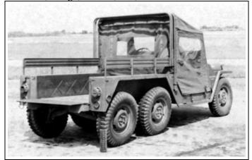
Vehicle Data: Length: 162 in (4115 mm). Width: 62 in. (1575 mm). Weight empty: 2450 lbs. (1112 kgs.). Payload: 1900 lbs. (862.5 kgs.). Engine: Gasoline, 4-cyl, 70 hp (51.7 kW). Transmission: Manual, 4F-1R. Tire size: 7.10 x 15.
