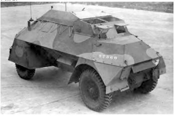
**Remarks**: The second version of the Australian Light Armored Car, Rover. The Mark 2 was shortened by some 24 inches (610 mm) but this didn't actually change the internal volume of the fighting compartment. An open topped vehicle; the Rover had a surprising amount of internal room for the crew and their gear.
