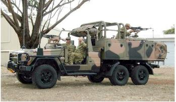
**Remarks**: Australian Army Mercedes-Benz G-Wagon 6×6 Surveillance Reconnaissance Vehicles (SRV) fitted with a locally fabricated custom weapons suite. Under Phase 3A of the projected vehicles on order, approximately 200 SRVs will receive front and rear weapon mounts.
