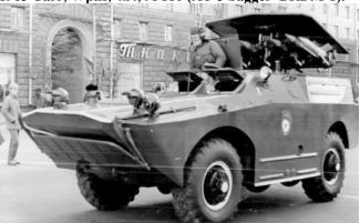
Above: Soviet/Russian 9P110 missile carrier during one of the yearly parades in Moscow. The launcher rails and cover had a limited left and right powered rotation to give some flexibility to placement of the vehicle. (Photo: Author's collection)
