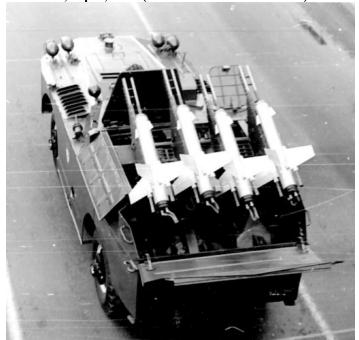
Above: Soviet/Russian 2P32 missile carrier. Fitted with powered (non-armored) cover panels, the covers could also be supplemented with a tarp to keep out the weather. (Photos: Author's collection)
