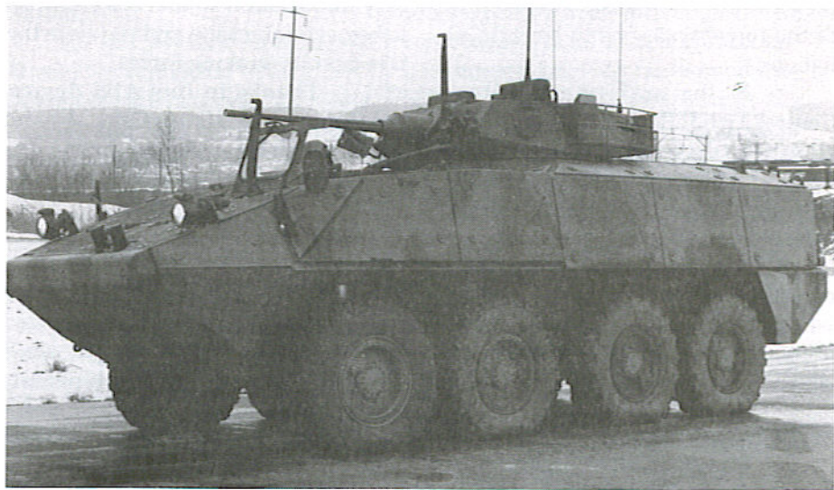
Above right: Piranha III (8x8) with its tires deflated. Note add-on armor and Delco turret. Photo: Raymond Surlémont. Below: Piranha 10x10 with 105mm NATO standard tank gun and GIAT TML turret during firing trials. Photo: MOWAG Motorwagenfabrik AG.
