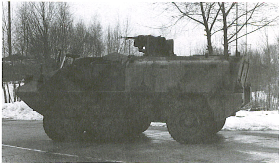
Above: Piranha III (6x6) with a provisional machinegun mount and shield. Photo: Raymond Surlémont.
