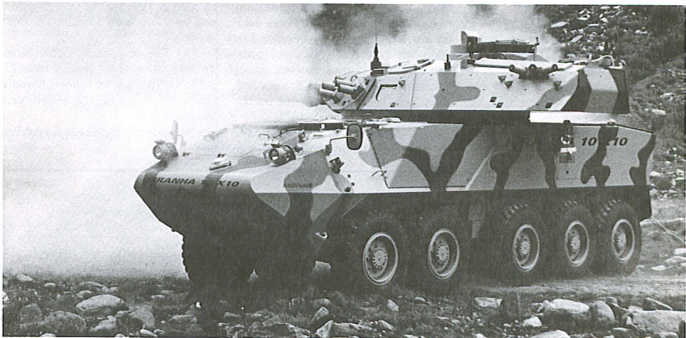
Above right: Piranha III (8x8) with its tires deflated. Note add-on armor and Delco turret. Photo: Raymond Surlémont. Below: Piranha 10x10 with 105mm NATO standard tank gun and GIAT TML turret during firing trials. Photo: MOWAG Motorwagenfabrik AG.
