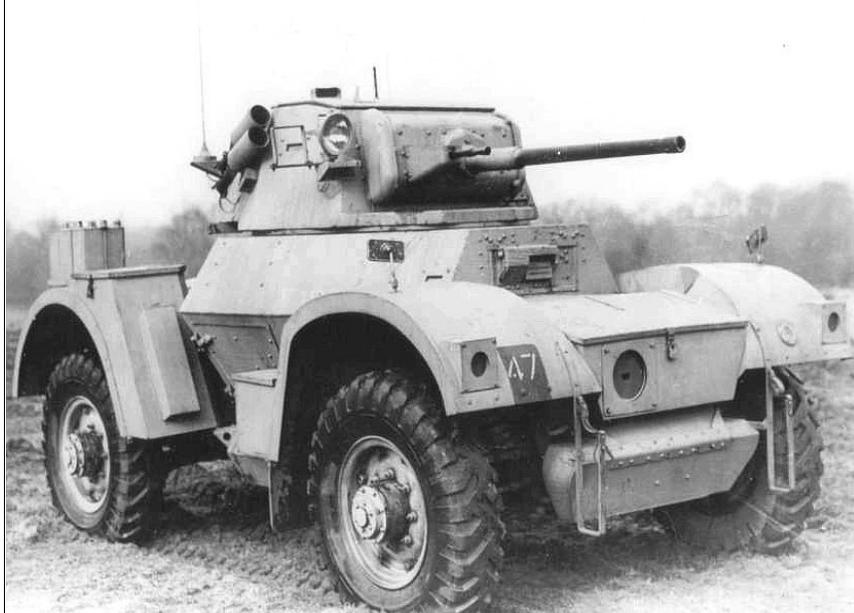
Above: Daimler Mk I armored cars, the lower photo shows a vehicle with spare gas cans known as “flimsies” mounted on the rear fender. The most obvious difference between the Mk I and Mk II is the rectangular mantlet of the Mark I.
