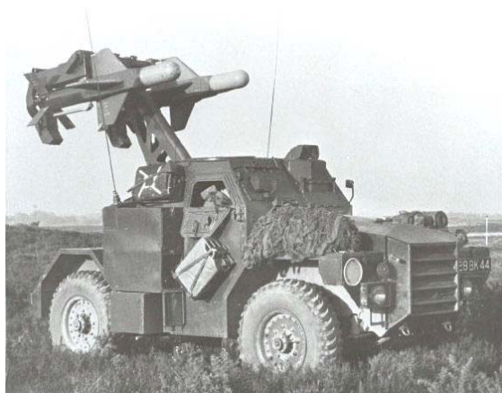
The early position of the upper jerrycan holder. Note the exhaust now goes to the front of the vehicle emerging just in front of the front wheel.
