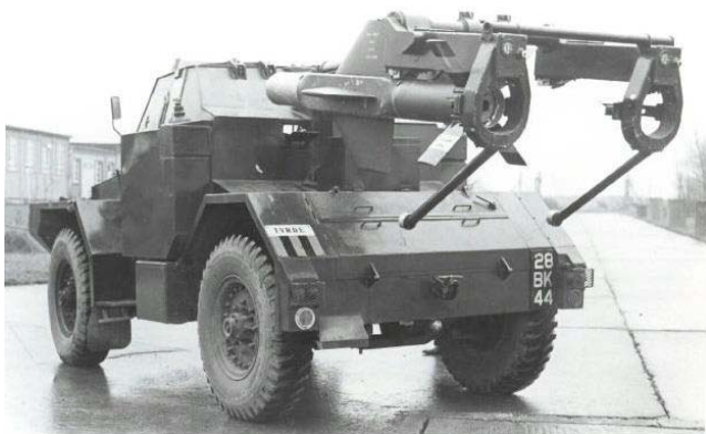
FVRDE prototype, note fixed wire dispenser arms and rear exhaust protection plate.
