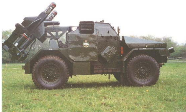
The later Hornet, which now has an armoured extractor fan, cowl in place of the upper jerrycan. Note locker on front wing – see text.
