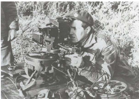
Intense concentration during training with the separation firing kit, in operational use the controller would be wearing a headset to give the order to fire the missile.
