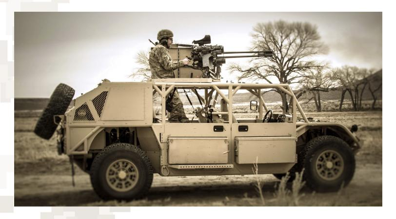
The Flyer® 72 is a non-developmental item, purpose-built, light-weight vehicle designed to meet complex mission sets. Selected by the U.S. Special Operations Command (SOCOM) as the vehicle of choice for their Ground Mobility I.I (GMV I.I) program, at 72" wide it is capable of internal transport in the CH-47 and C-130 aircraft.
