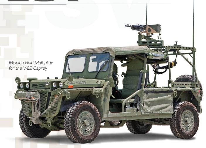
The Light Strike Vehicle (LSV) is an air-certified ground mobility platform for the V-22 Osprey Tiltrotor aircraft. A member of the family of Internally Transportable Vehicles (ITV), the LSV offers unmatched safety, agility, mobility and payload capacity in a compact space envelope. Internal transportability allows US forces to take full advantage of the 270 knot forward air speed of the Osprey transporting internal loads.
