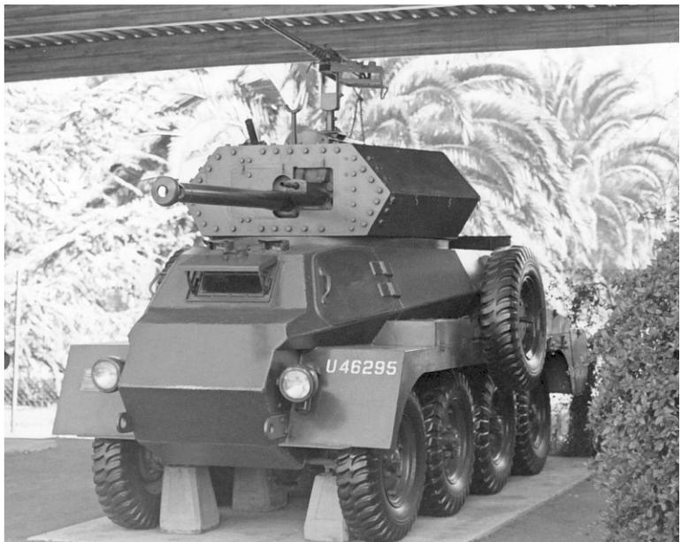
*Remarks:* After the Mk V, came the Mark VI, another eight wheeled vehicle, but of lighter design. Of the two prototypes completed, the first mounted a 2-pdr (40mm) gun, and the second a 6-pdr (57mm). By 1943 work on the Mk VI had progressed to a second prototype, but the pressing need for armored cars had diminished. The British order for 250 cars was canceled and development continued at a slow pace, only the two original prototypes were actually com-
