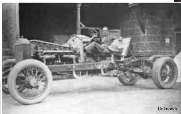
Rolls-Royce 40/50 "Alpine Eagle" chassis prior to armoring circa 1914. Note dual rear wheels, additional spring leaves, and auxiliary fuel tank behind fire-wall.
