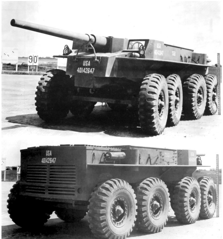
Above and left: The single T55E1 during testing at Aberdeen Proving Ground. The E1 was made of mild-steel, rather than armor plate. (Photos: US Army)
