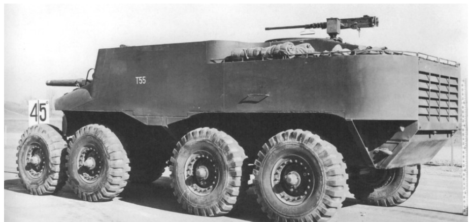
Above: The rather complicated T55 design was replaced by a more angular version in the T55E1; neither was selected for production. (Photos: US Army)
