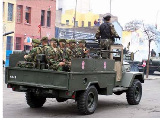
Above: Peruvian Army M-325 with "B" body set up as a personnel carrier with seats facing out and mounts for light machine guns. (Photo: Peruvian Army).
