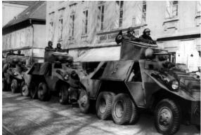
**Remarks**: Welded armor plate, three heavy machine guns and two light. 20'6"x6'10"x8'2".
