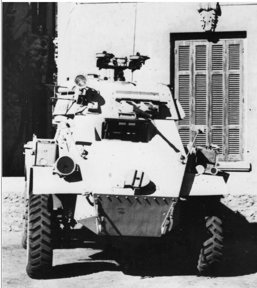
Above: Two views of Humber Armored Car(s) Mk III one of which is fitted with twin Vickers machine guns.
