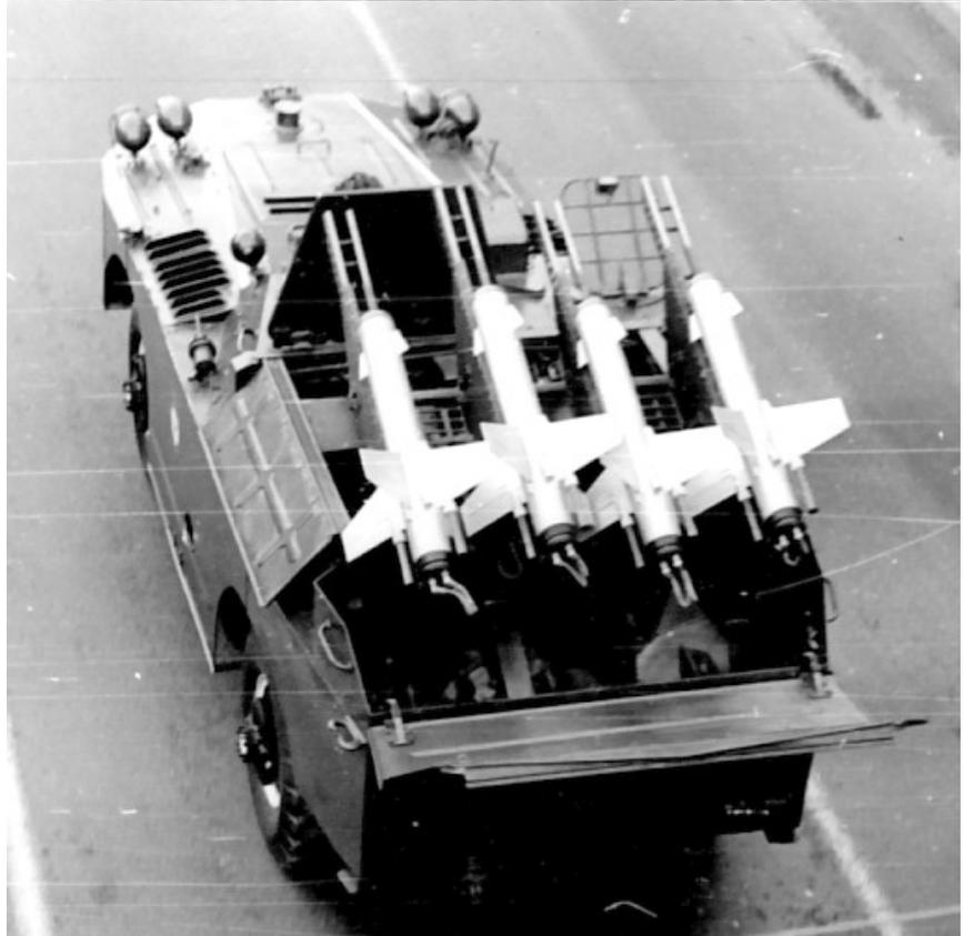
Above and top: Soviet/Russian 2P32 missile carriers. Fitted with powered (non-armored) cover panels, the top could also be supplemented with a tarp to keep out the weather. (Photos: Author's collection)
