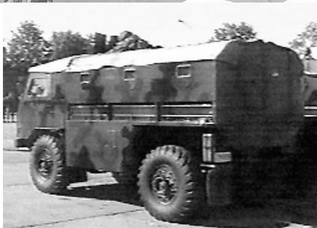
Above: Two views of the TAM 110 Ris (Lynx) Armored Personnel Carrier. The vehicle can be fitted with a light or heavy machine gun and firing ports are supplied under the side vision windows, a separate firing port is also available under the right hand windshield. (Photos Tovarna Avtomobilov Motorjev [TAM])
